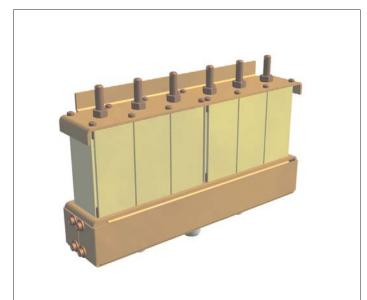
The helical duplexer HDF166.Q34 is a symmetrical duplexer made of six High Q helical resonators in a Band-reject configuration. The duplexer is designed for the operation of the transmitter and receiver together in to one antenna in bands of 140-180 MHz.
