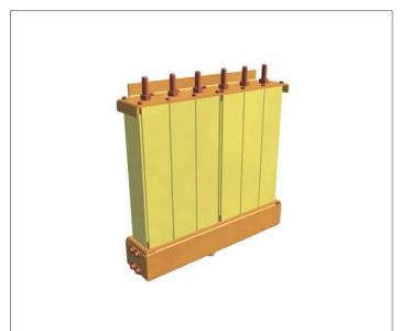
The helical duplexer HDF456.Q34 is a symmetrical duplexer made of six full-lenght  $1/4 \lambda$  resonators in a Bandreject configuration. The duplexer is designed for the operation of the transmitter and receiver together in to one antenna in bands of 440-470 MHz.
